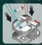
Place the tip of an explorer 1 into the clip's easily accessible circular opening or 2 at the end of the clip's alignment quide
